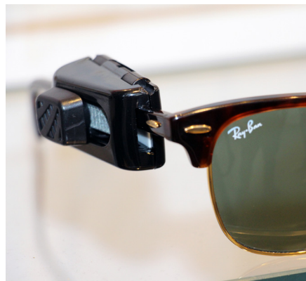
The F-117 Nighthawk was designed to tighten its grip in the event of an improper removal.
